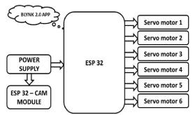
**ESP32 Microcontroller:** The ESP32 microcontroller is the main processing unit in this robotic arm system. It is a powerful and versatile microcontroller with built-in Wi-Fi and Bluetooth capabilities, making it ideal for IoT applications. **Controlling Servo Motors**: The ESP32 generates PWM (Pulse Width Modulation) signals to control each of the six servo motors.
