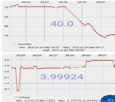
Fig A.1 Humidity & Voltage
