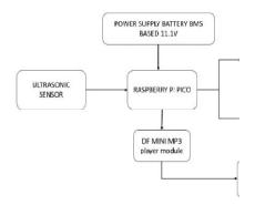
The system uses an ultrasonic sensor for obstacle detection, a GPS module for location data, and a GSM module for communication. The system outputs audio files to the DF Mini MP3 Player and speaker, with the ultrasonic sensor triggering an audio alert based on the object's distance.
