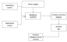
The system uses a distributed processing model with two NodeMCU ESP8266 microcontrollers for optimal performance and reliability. It consists of three primary components: sensor nodes for physiological data, Firebase for data storage, and a mobile/web application for caregivers. The MAX30100 Pulse Oximeter is a medical device that is used to measure blood oxygen saturation levels, heart rate, and pulse strength. It uses a non-invasive method to measure oxygen saturation levels in the blood.
