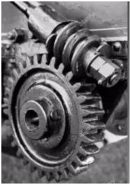
The rotary motion of worm is converted in to the angular movement of drop arm.
