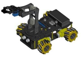
After successful testing and calibration, the final robot is deployed for real-world tasks. The ESP32 controller, high-torque servo motors, mobile base, and robotic arm are all integrated into a cohesive system capable of performing autonomous navigation and manipulation.
