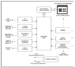
**PH sensor :** A PH sensor is used to detect the pH value of water, determining whether it is within the safe drinking range (pH 6.5-8.5) and indicating if the water is drinkable or not.
