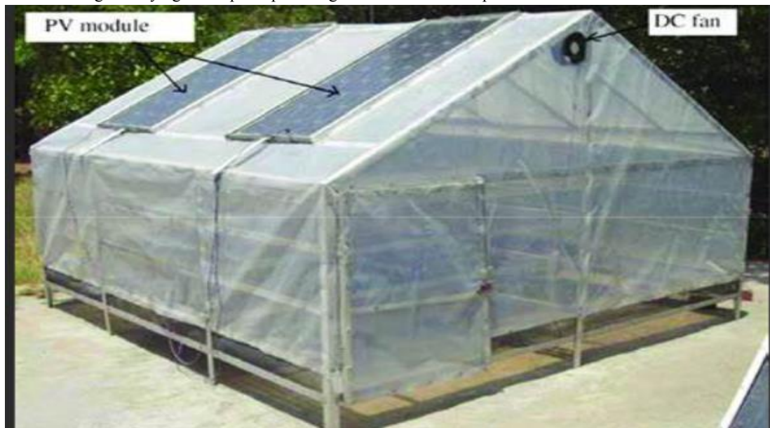
Fig. 2- Setup-of greenhouse-dryer-operating-under-active-mode-Barnwal-and- Tiwari-2008
