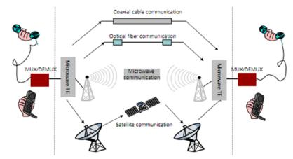
The two types of microwave transmission are terrestrial and satellite: Terrestrial microwave transmissions are sent between two microwave stations on the earth (earth station). It is the most common form of long-distance communication.
