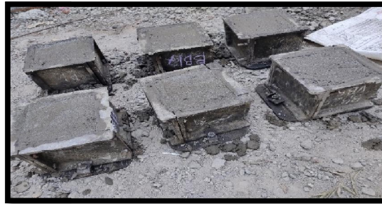
Fig. 2. Casting of Cubes
