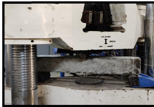
Fig. 3. Test Setup of flexural beam for one point loading
