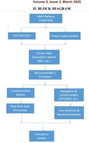
UMV Platform: UAV (Unmanned Aerial Vehicle) or UGV (Unmanned Ground Vehicle) as the physical platform for gas detection.
