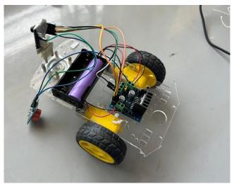
MODULE contain front camera live image or video capturing it can see in mobile screen. It contain gas leakage sensor to sense gas leakage. It give alter notification on mobile.
