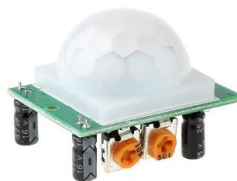
Fig. 6. PIR Motion Sensor
