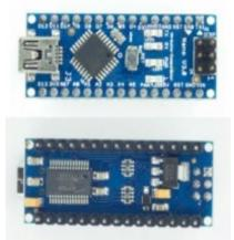
It lacks only a DC power jack, and works with a Mini-B USB cable instead of a standard one. The Arduino Nano can be powered via the Mini-B USB connection, 6-20V unregulated external power supply (pin 30), or 5V regulated external power supply (pin 27). The power source is automatically selected to the highest voltage source.
