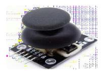
This is JoyStick Module PS2 Breakout Sensor very similar to the 'analog' joysticks on PS2 (PlayStation 2) controllers. Directional movements are simply two potentiometers – one for each axis. Pots are  $\sim$ 10k each. This joystick also has a select button that is actuated when the joystick is press down.
