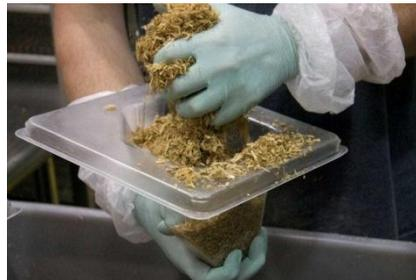
The material obtained from fungi's mycelium grown in a mould – whose growth is interrupted through heating and dehydration at the end of the biochemical transformation – is inert and free of spores Ecovative .
