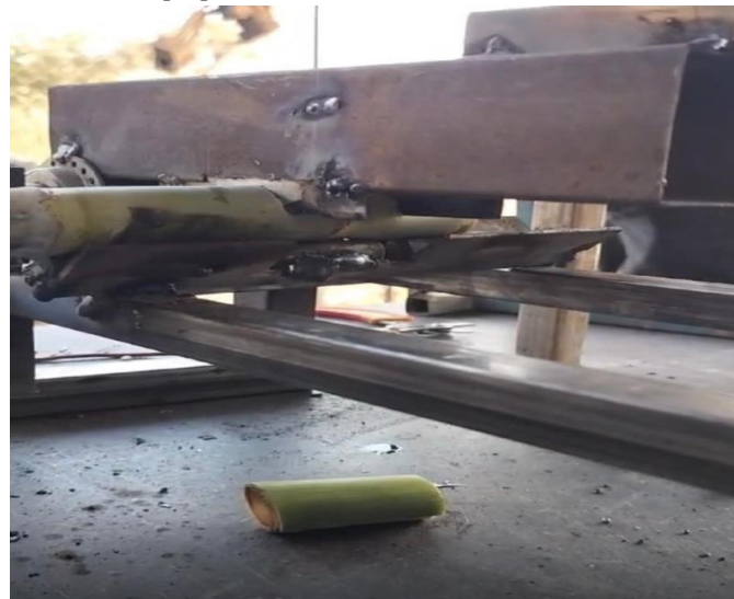
Fig 3.4 Testing of Sugarcane bud cutter machine
