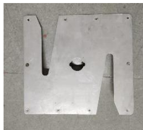
FIG. 5.1 CUT TIN METAL SHEET BY USING LESER CUTTING
