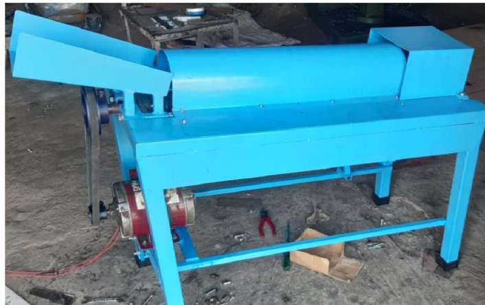
Fig. 1.2 Corn thresher machine
