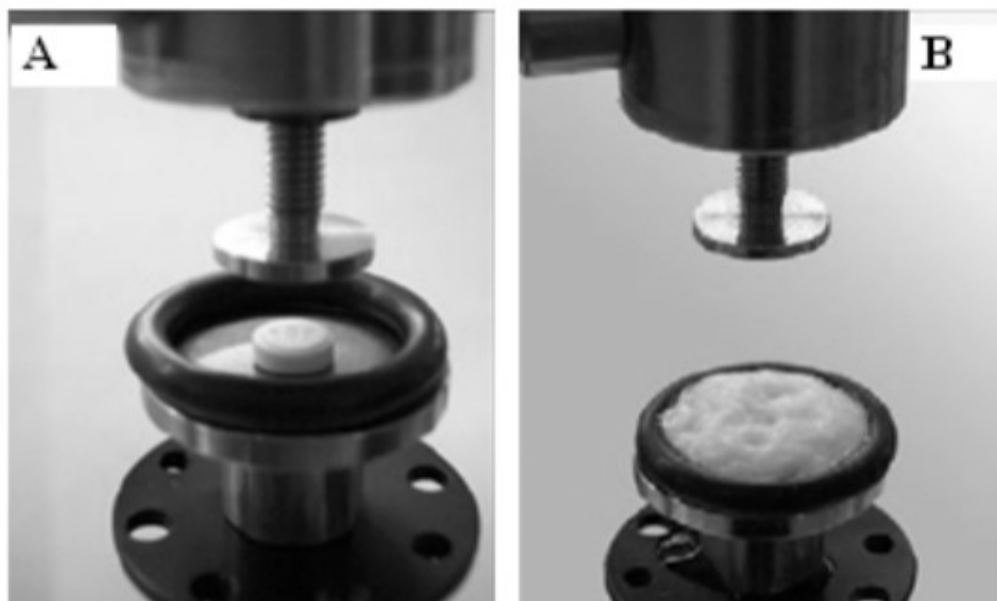
Fig.14. ElectroForce® apparatus for Disintegration test A. ODT mounted on test plate before loading. B. ODT after completion of Disintegration test
