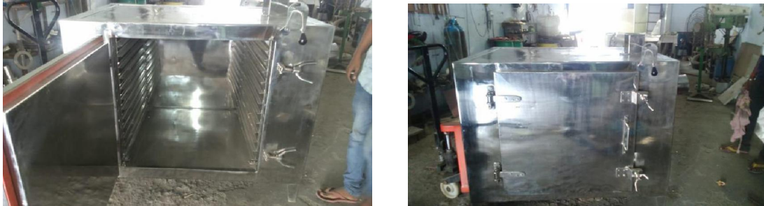
Figure 4: Assembled Tray Dryer Undergoing Final Testing
