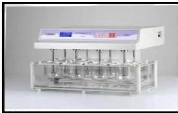
Fig No. 5 Paddle Method in Dissolution Apparatus
