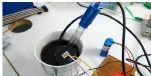
Fig: Testing water quality in real time by mixing solvents in water
