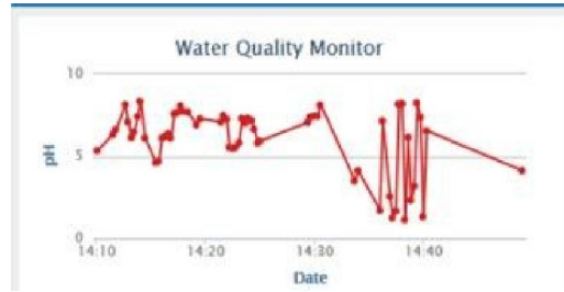
Real time visualization of pH variation in water sample
