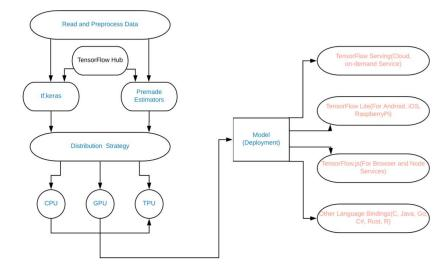
**4. Distribution Strategy:** Since object detection in a Realtime blind-assistance system requires fast and efficient processing: CPU: This may be sufficient for simple, lightweight detection. GPU: For faster object detection processing, especially when real-time feedback is needed. TPU: Could be beneficial for optimizing real-time detection, especially for handling complex environments.
