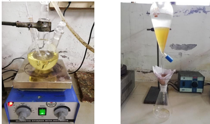
Figure 4: (a) Synthesis of Glycidyl acrylate and (b) Washing filtration
