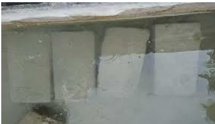
Figure: Experimental setup for Water Absorption test
