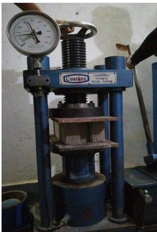
Figure: Experimental setup for Compression Test
