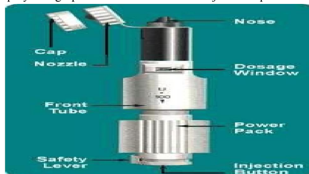
Detailed Diagram of insulin jet injector
