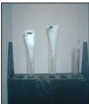
Fig-2: The sediments filtering method in laboratory Copyright to IJAR SCT www.ijarsct.co.in
