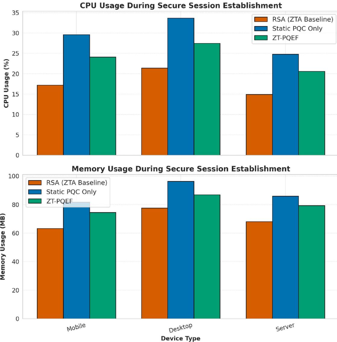
**Figure 5. CPU and Memory Overhead During Post-Quantum Handshakes**
