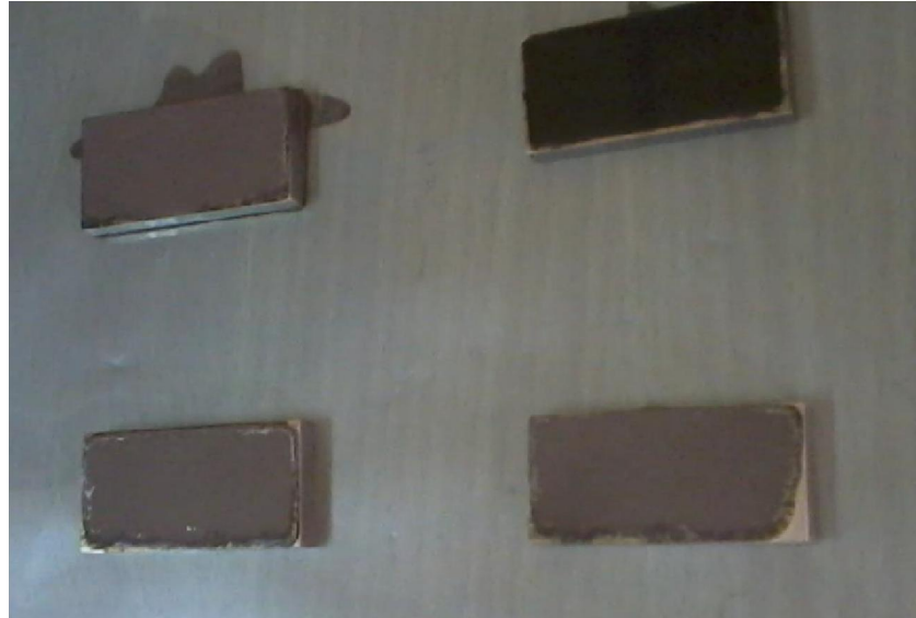
Fig 3 AISI 304 Steel samples after preplacing of TiC powder
