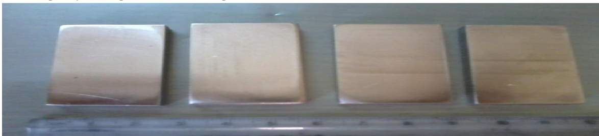
Fig 2 AISI 304 Steel samples prior to coating
