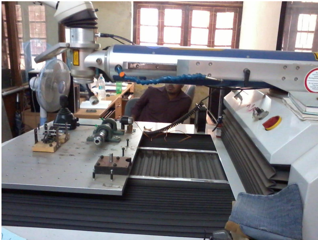
Fig 4. Nd-Yag pulsed laser experimental setup for development of coating
