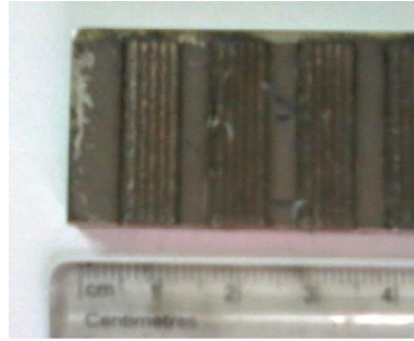
Fig 6-After coated sample of AISI 304 steel
