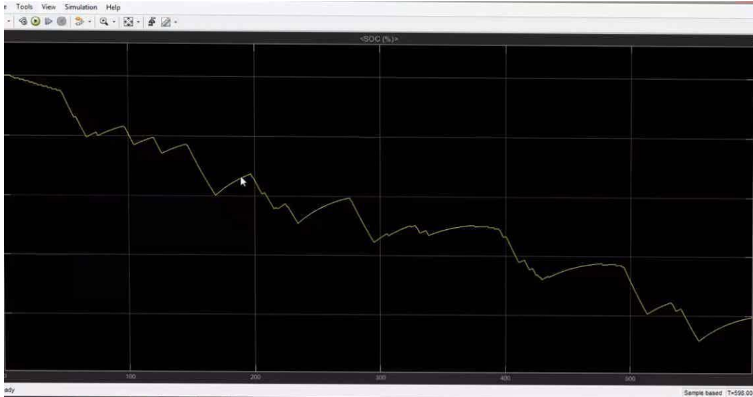
Fig. 6. State of charge variation due to Regenerative braking.
