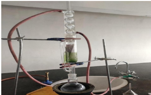
Fig 6 :Extraction of Vincristine and Vinblastine via soxhlet apparatus
