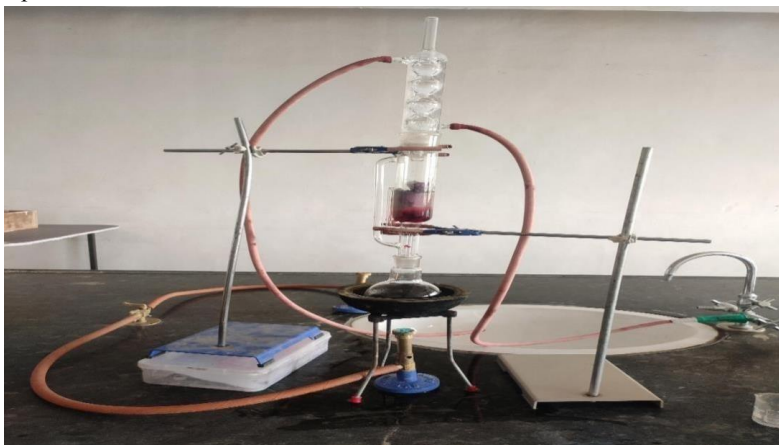
Fig 5: Extraction of hibiscus via soxhlet appratus
