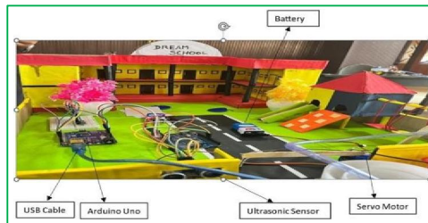
Figure 7: (Ultrasonic Sensor using Servo Motor working image)
