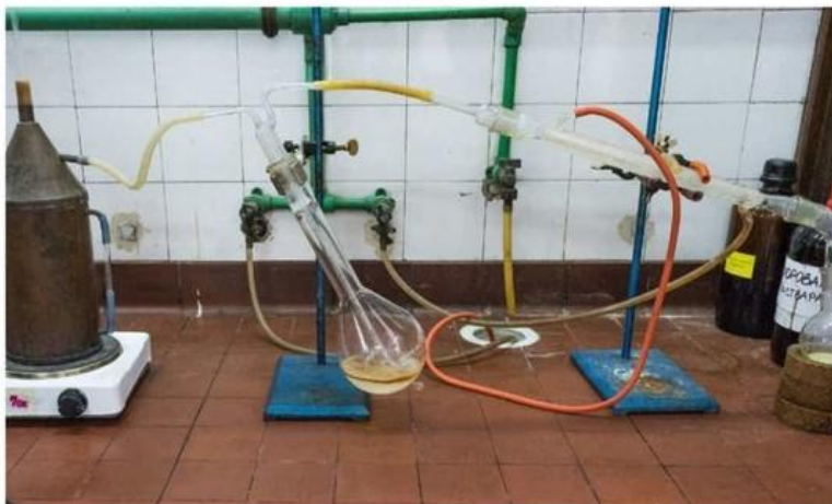
FIG NO 5 : Process Of Steam Distillation
