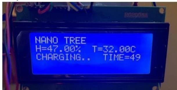
Fig 4. Weather forecast details and charging duration are shown on the LCD screen
