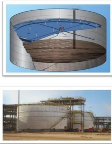
Figure 2: Fixed pressure type tank
