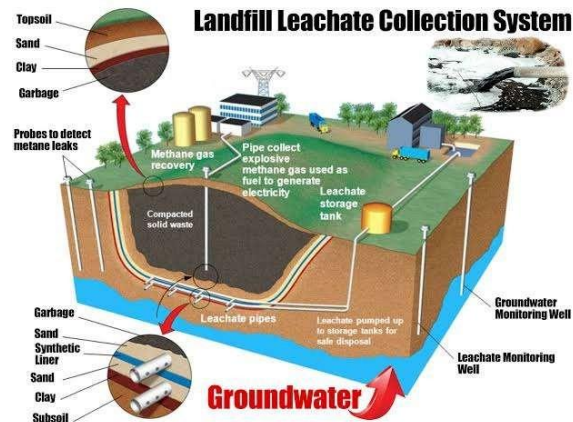
Fig 1: Formation of Leachate in Landfill Site
