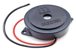
This is a Small PCB Mountable 3V Active Electromagnetic Buzzer. It is great to add Audio Alert to your electronic designs. It operates on 3V supply, uses a coil element to generate an audible tone.
