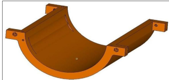
Fig. 2.1 One half of split type journal bearing [2].
