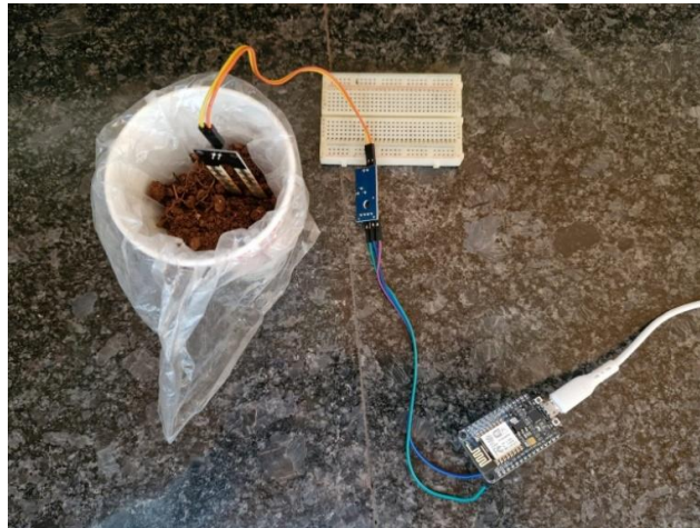
Fig 6.1.1 Moisture sensor connection
