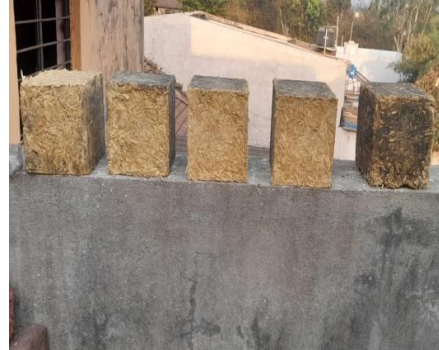
After unmould cubes are open dried for 28 days
