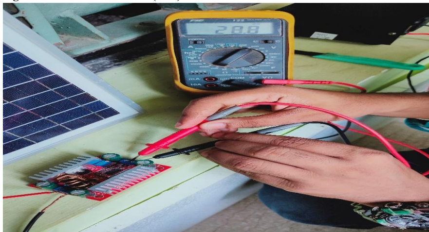
Figure 10: Output voltage test of DC-DC boost converter with multimeter
