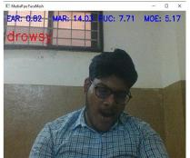
Fig: 7.3 Drowsy Due to Eyes are Closed
