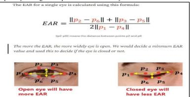
Fig: 6.1 Eye Aspect Ratio with Facial Landmarks
