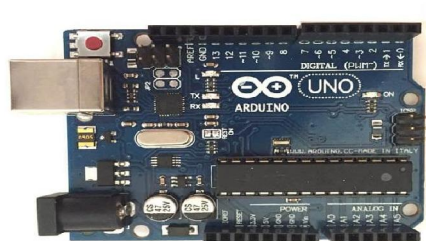
Figure 7: -Arduino with ATmega328P microcontroller
