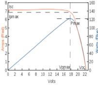
Most solar panels produce much higher voltage than is necessary to charge a 12V battery, or 24 or 48 volts if you have that configuration. A 12V charging panel will actually produce 16 to 18 volts, depending *m* conditions, but only about
