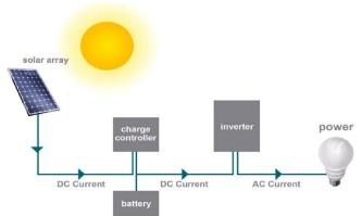
It ensures that the battery is not overcharged or undercharged, which can damage the battery and reduce its overall lifespan. The solar charge controller also prevents the battery from discharging back through the solar panel at night. It is a critical component in a solar power system. The Solar Power can be measured using Pranometer Sensor.
