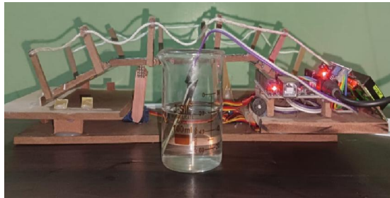
Fig:1.3 Soil Moisture Sensor Detecting Increased Water Level
