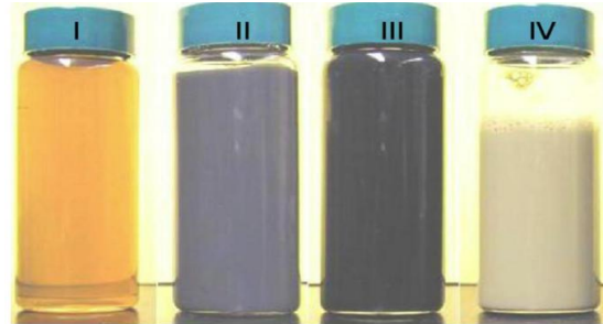
Fig.4. Typical samples of Ag-deionized nanofluids generated by multi beam ablation in liquid technique [119].
