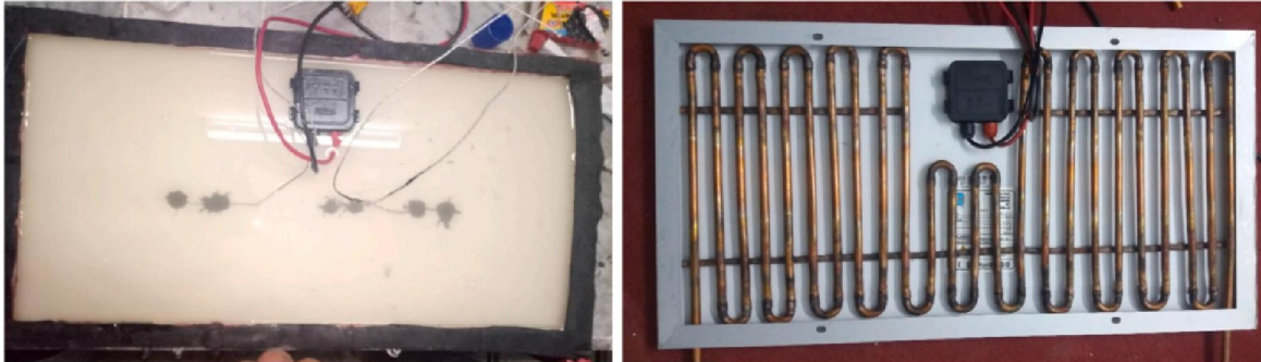
Fig. 5. (a) Molten paraffin wax filled in Al container; (b) Cu tubes serpentine channel networks inside PCM box.
