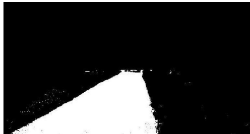
Fig. 3. The detected road surface
