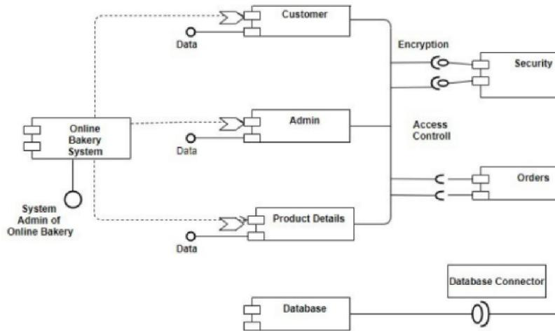
Fig.5. Component Diagram
