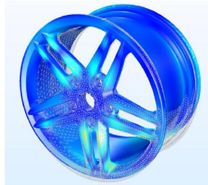
**Finite element discretization, stresses, and deformations of a wheel rim in a structural analysis**
