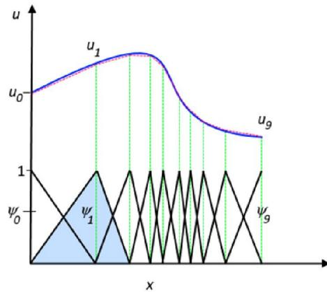
The function  $u$  (solid blue line) is in line with  $u_h$  (dashed red line), which is a linear combination of linear basis functions ( $\psi_i$  is represented by the solid black lines). The coefficients are denoted by  $u_0$  through  $u_7$ .
