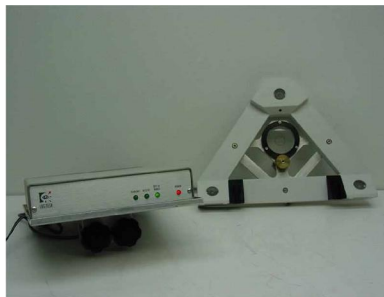
Fig: 5 Logitech ultrasonic tracker
