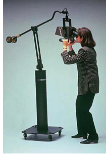
Fig: 3 A Binocular Omni-Orientation Monitor (BOOM)
