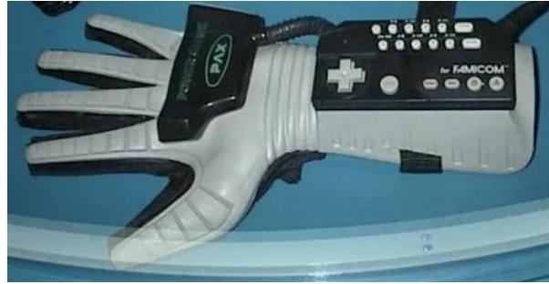
Fig: 6 An instrumented glove (Nintendo power glove)
